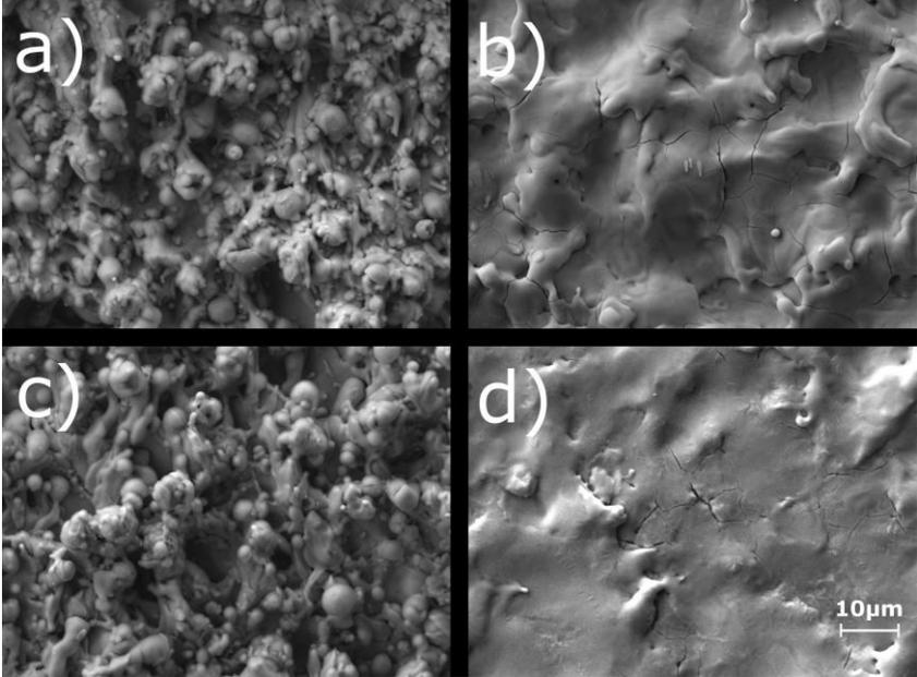
**Fig. 3** SEM images of modified samples surfaces at a magnification of 1500 x: a) sample C; b) sample W1; c) sample O1; d) sample O3
