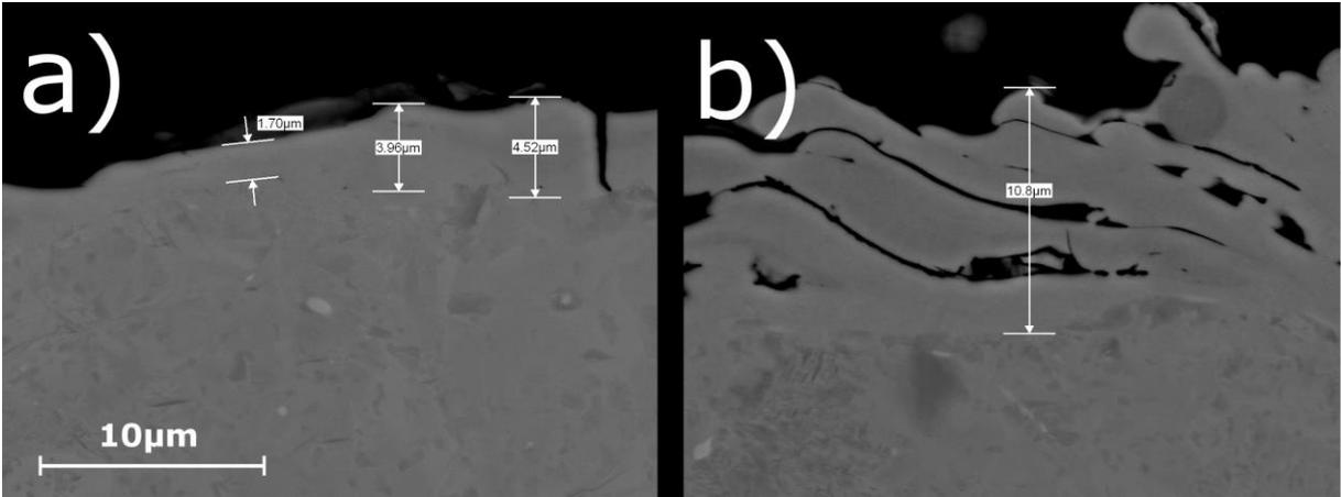
*Fig. 6 Heat affected area: a) sample W1; b) sample O1*
