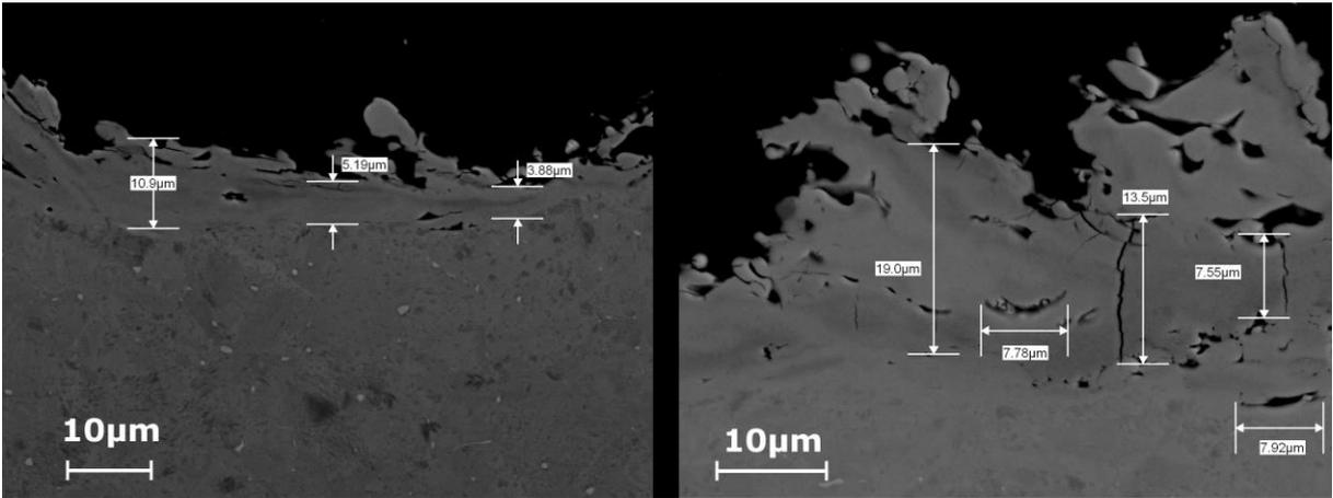
*Fig. 5 Heat affected area of sample C in different scale*
