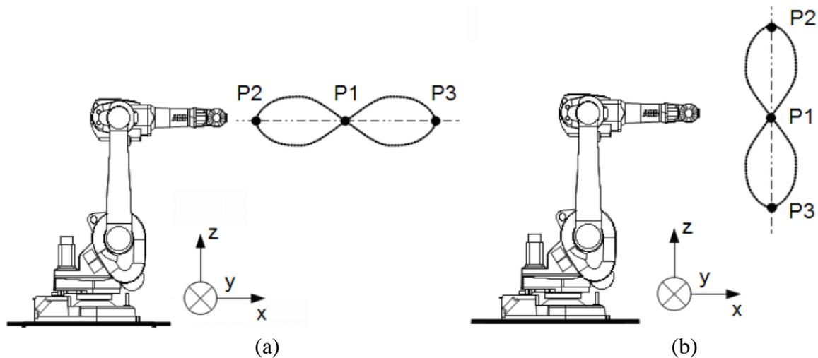
**Fig. 3** Investigated trajectory – (a) horizontal movement (b) vertical movement [20]
