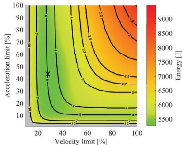
**Fig. 2** Energy consumption (colour map) and motion time (isolines) as function of velocity and acceleration limits [22]
