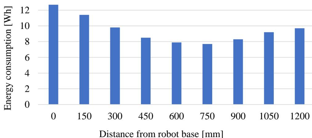
**Fig. 1** Graph of energy consumption depending on the height of the product [20]
