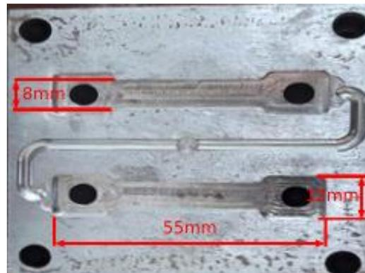
*Fig. 1* Cavity of used mould
