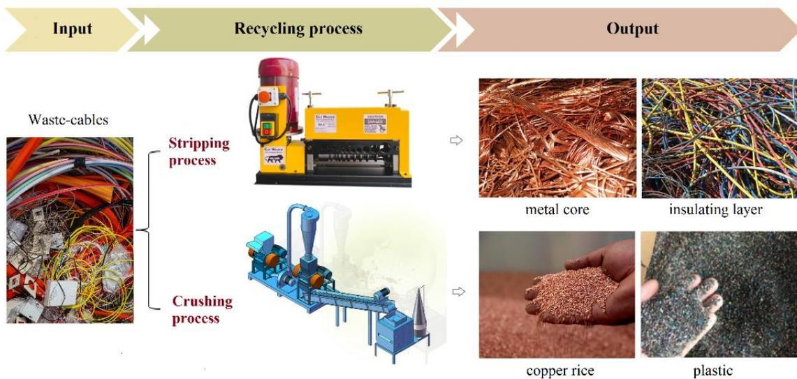
**Figure 1** Mechanical treatment technology of cables (stripping and crushing process). Adapted from [92-96].
