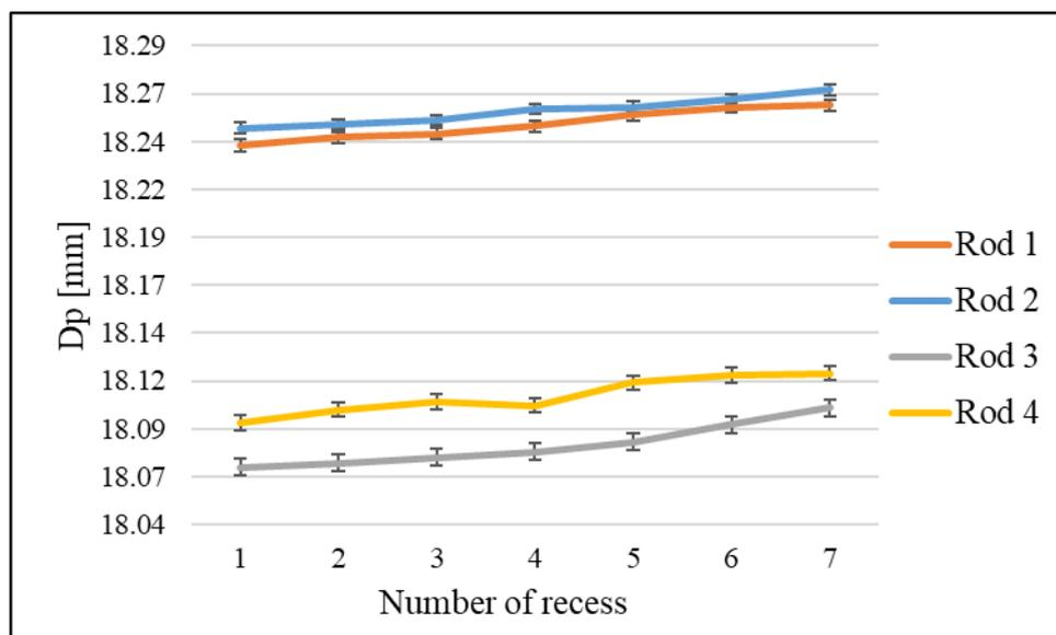
**Figure 6** Diameter of recesses after machining
