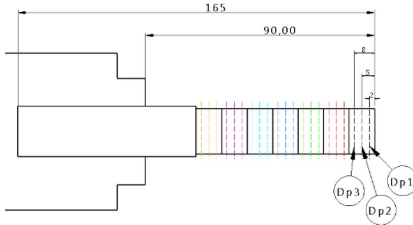
**Figure 4** Diameter measurement points
