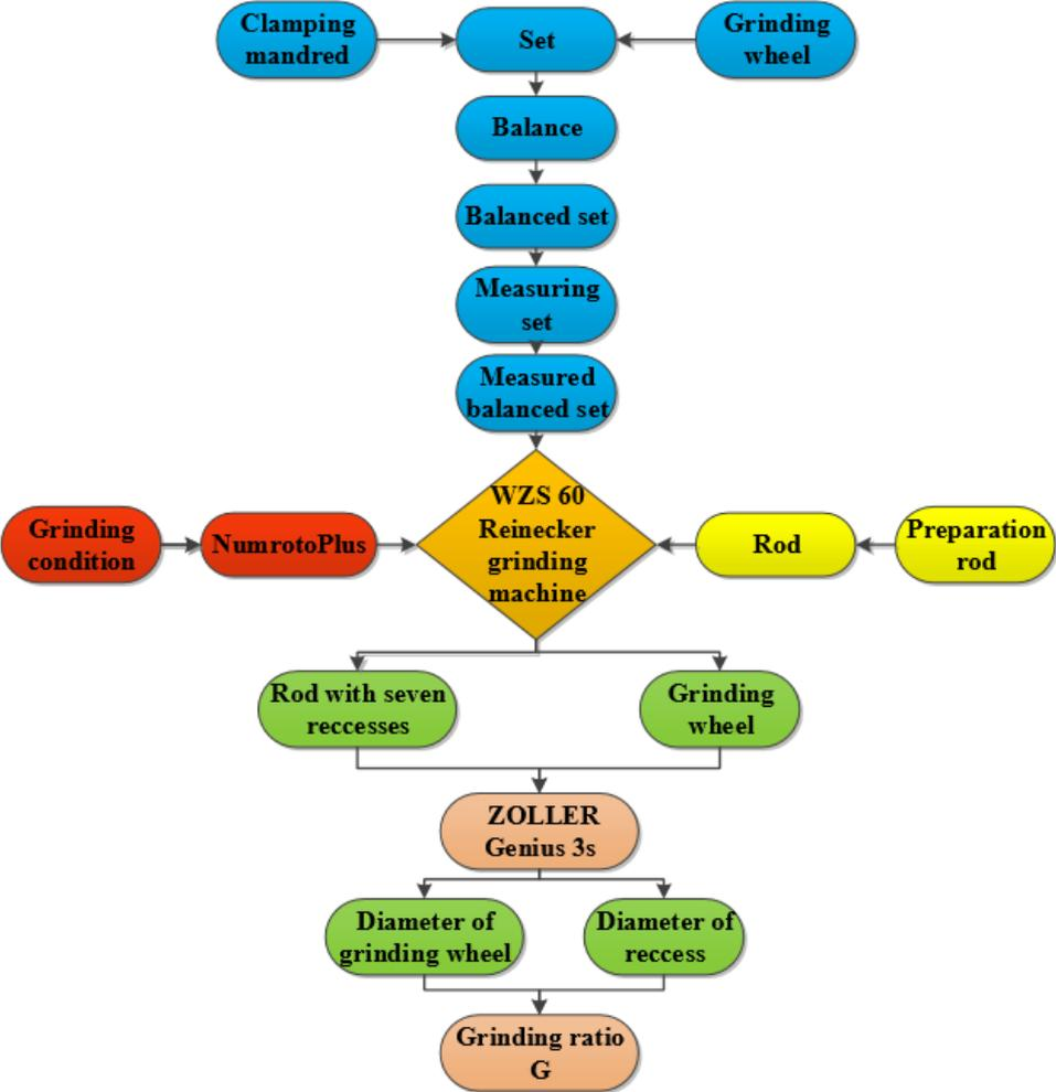
Figure 1 Scheme of the experiment implementation
