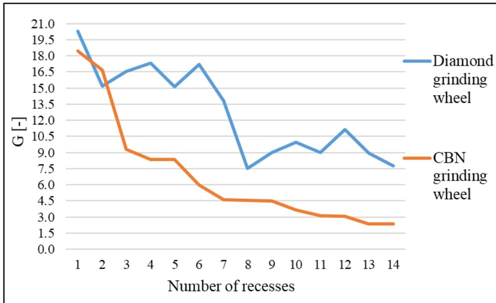
**Figure 5** Grinding ratio of diamond wheel and CBN wheel
