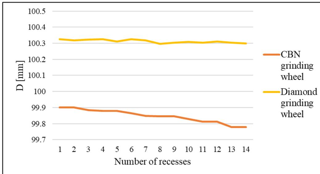
**Figure 7** The diameter of grinding wheels as a function of the number of recesses
