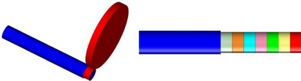
*Figure 2 a) The grinding of the first recess b) seven recesses after 3D grinding simulation*
