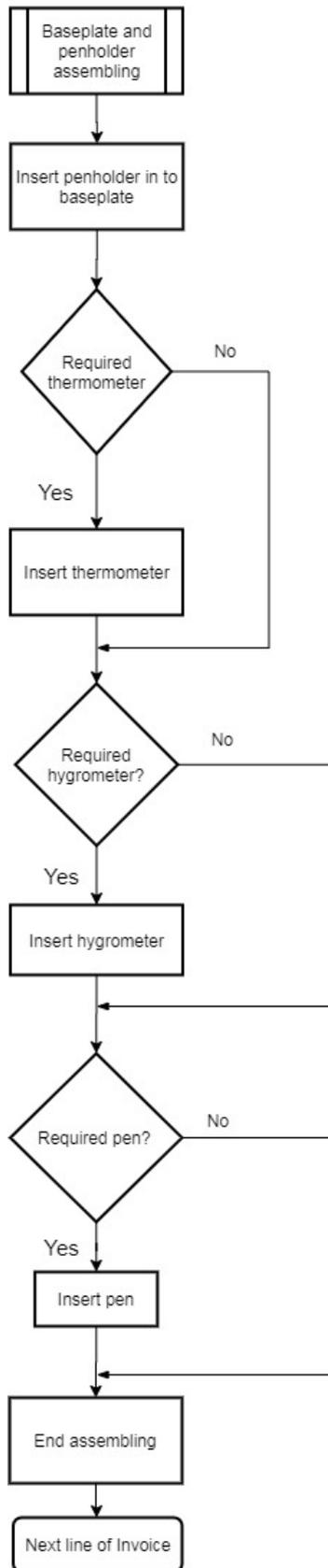
*Figure 5 Flow chart of production process in iCIM 3000*
