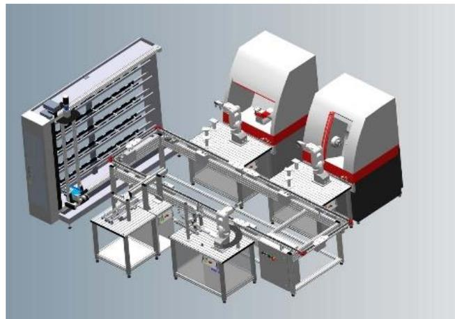
**Figure 2** Flexible manufacturing system of iCIM 3000
