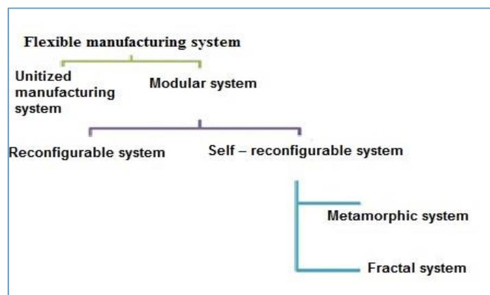
*Figure 1 Classification of flexible manufacturing systems*
