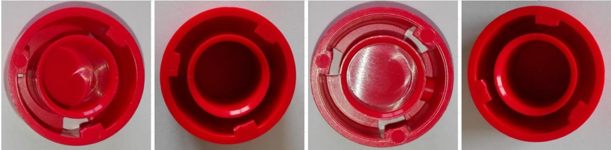
Figure 2 Example of recorded pictures of piston body from top – different lighting conditions
