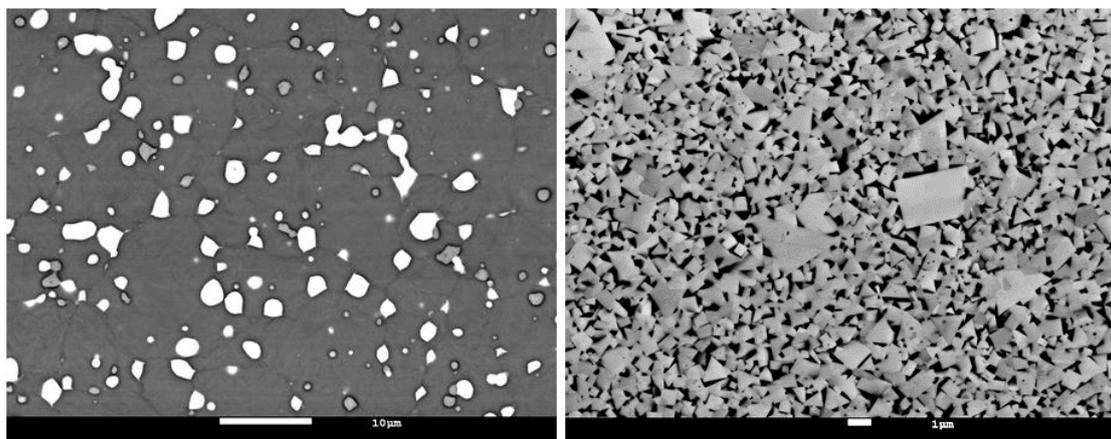
*Fig. 1 Microstructure of the substrates a) HSS, b) WC-Co*
