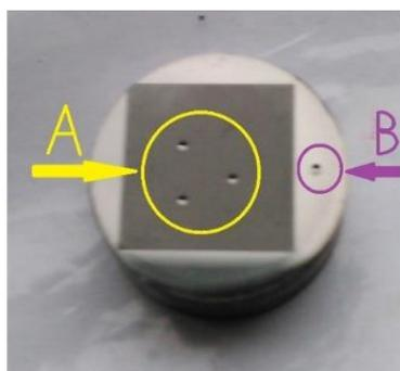
*Fig. 2 A - indent in the treated area, B - indent in the non-treated area*
